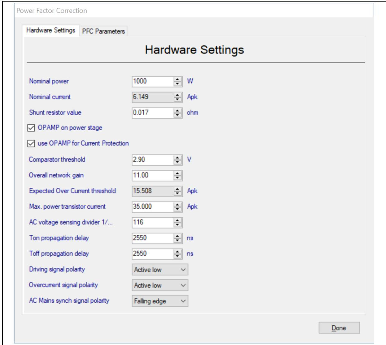
Figure 57. ST MC Workbench - Power Factor Correction GUI (PFC Parameters)
