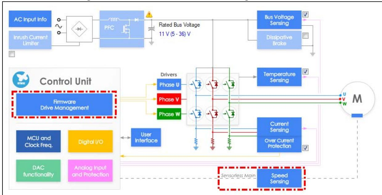
The following figures detail the Speed/Position Feedback Management GUI, where the user selects and configures the sensor(-less) as the main one, and eventually the auxiliary as another one, measuring the motor speed or position.
