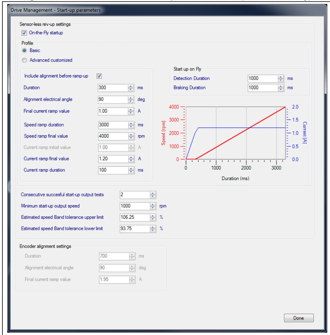
Figure 68. ST MC Workbench – Start-Up Parameters GUI (Advanced Rev-Up)
