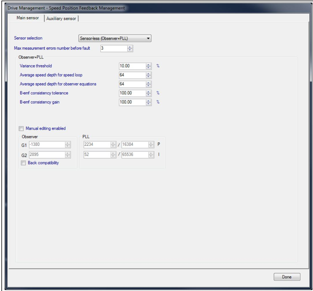
**Figure 60. ST MC Workbench – Speed/Position Feedback Management GUI (Sensor-less using Luenberger observer + Cordic)**
