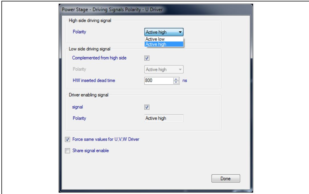
*Note:* The user can easily force the same settings for all three power drivers by ticking the “Force same values for U, V, W Driver” checkbox.
