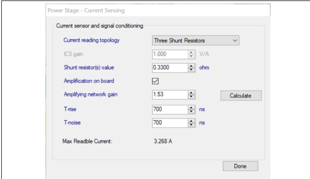
Figure 50 shows the *Amplifying Network Gain Calculator* GUI where the user configures the sensing implementation topology and related values.
