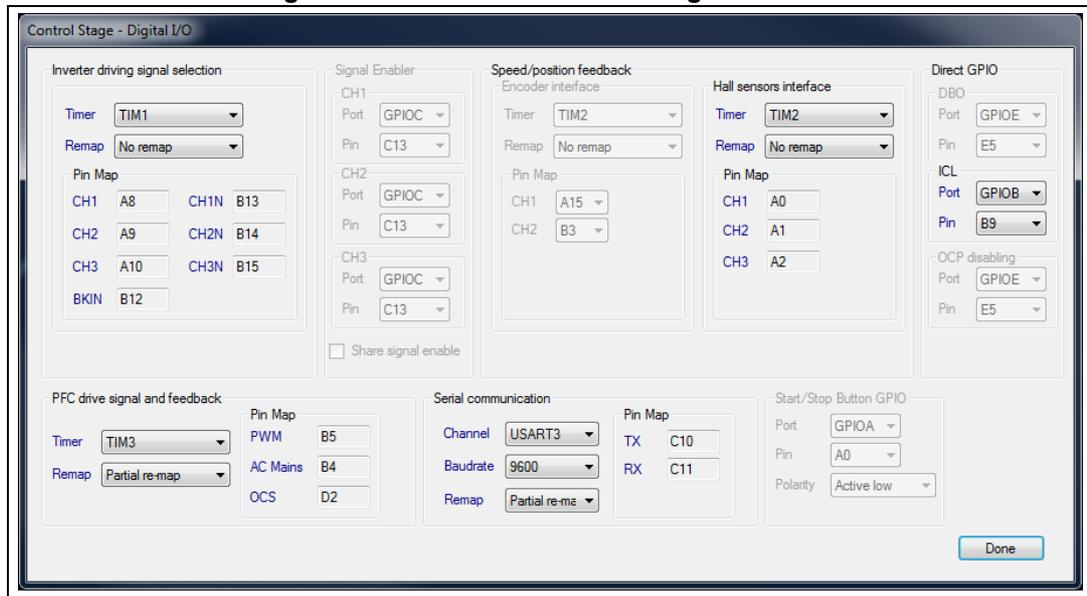
Figure 80 shows the User Interface Add-on GUI, where the user configures the interface for the control board usage: LCD (if supported), a Start/Stop push-button, and/or the serial communication link with software application.
