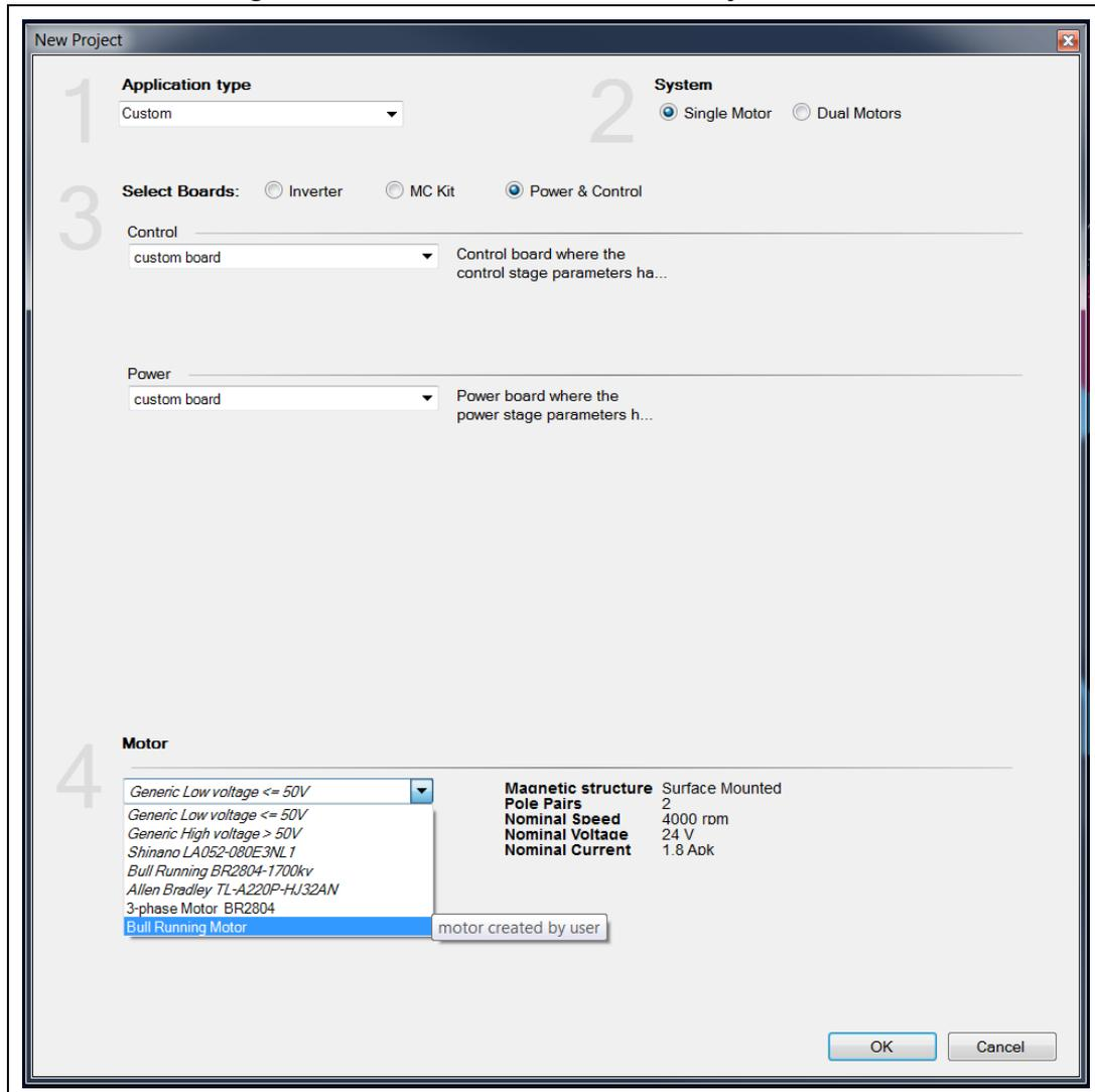
The created project imports the hardware settings according to the selected boards and motor profiling results. It also imports other settings like the PWM frequency and the startup acceleration used during motor profiling.
