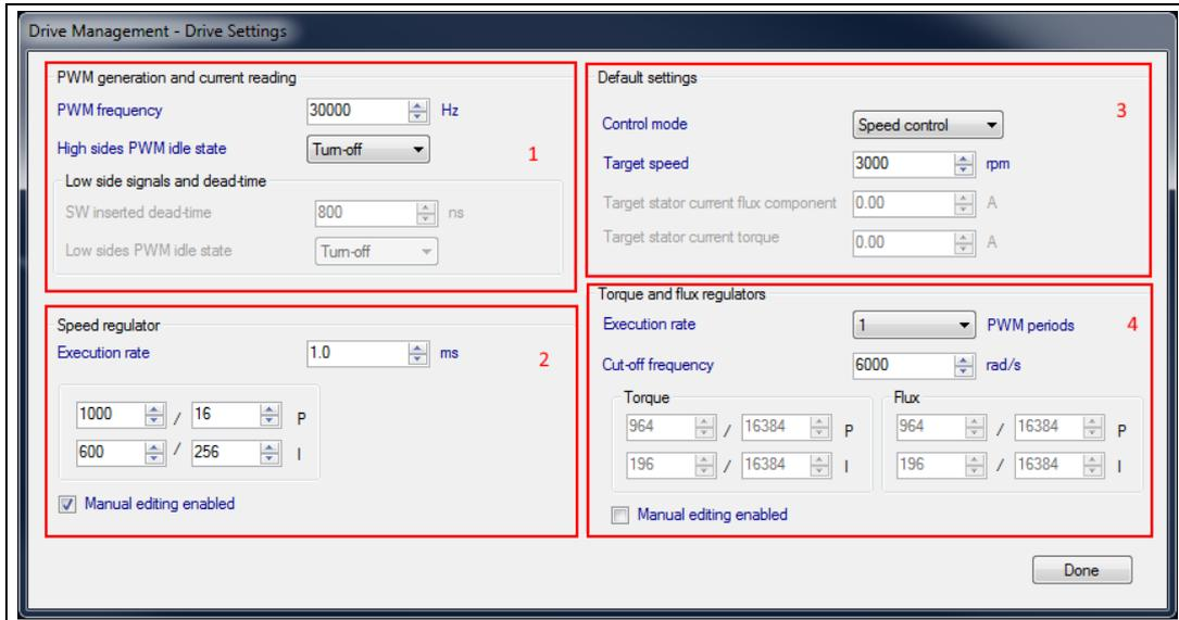
The PWM frequency is used to drive the power switches, while the PWM idle state for High and Low sides are usually Turn-Off (area 1).
