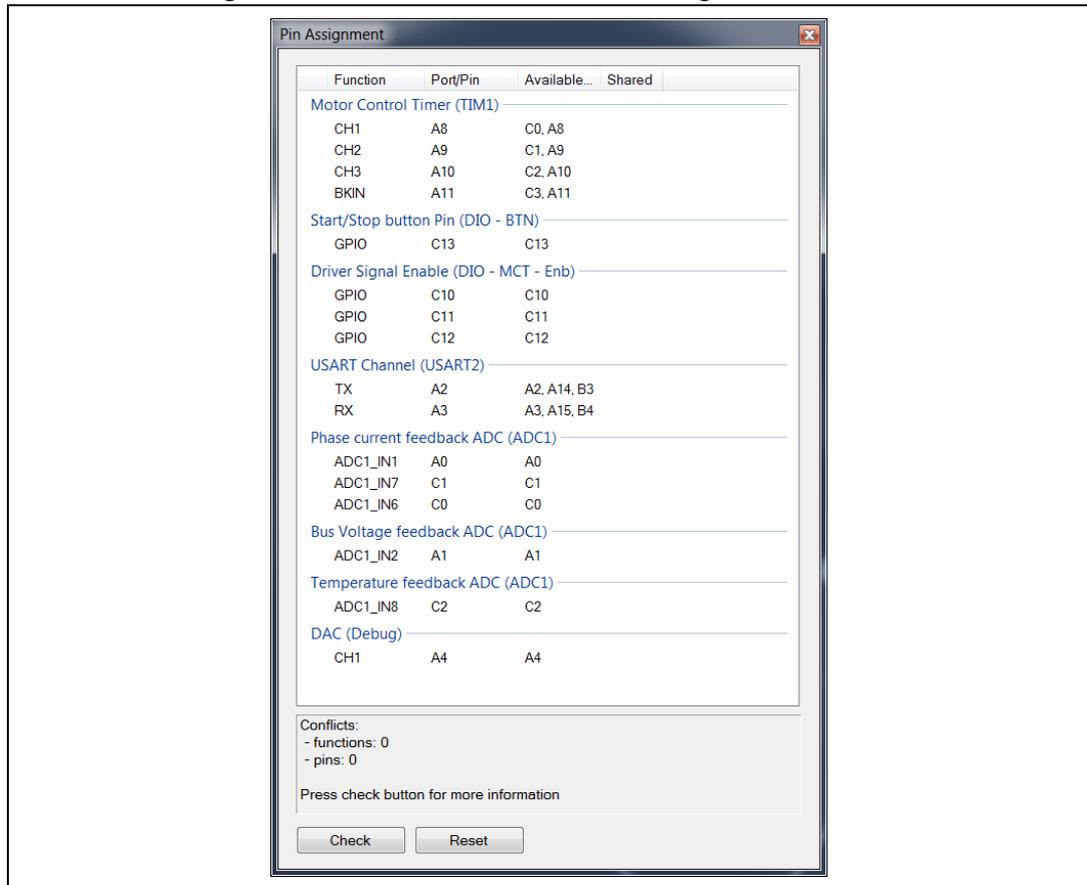
Figure 28. ST MC Workbench - Pin Assignment check window
